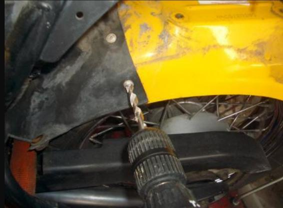
If you have a legend or later Thunderbird you will need to bolt on the seat catch, the holes are already present. Feed the cable down the side of the sub-frame and fix with cable ties so you can pull the nipple to release the seat
