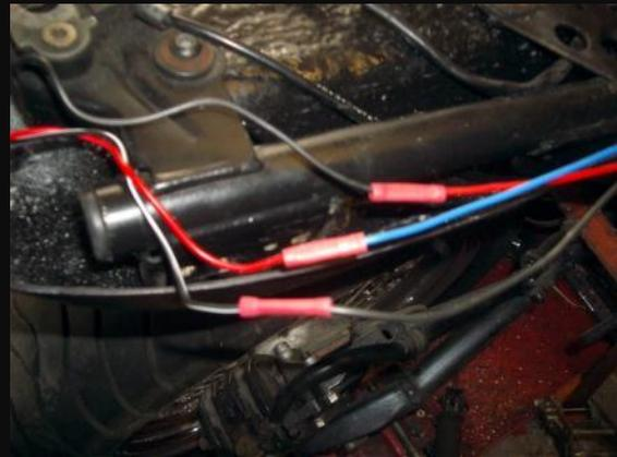
If using LED indicators bear in mind that they only work one way, so if they don't work swap the wires around. If using the original "bulb" indicators at the front and LED's at the rear you will need to fit a special flasher unit to get them to flash at the correct speed.
