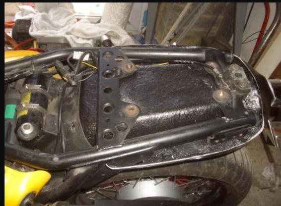
Pop the solo seat on to check the positioning and adjust by drilling out the holes on the eliminator slightly if necessary.
